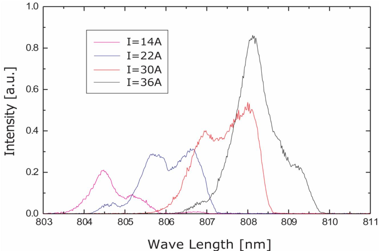
Emission spectra of high power laser diode P1202 of Coherent, Inc. for different values of diode current at constant temperature 20° C.
