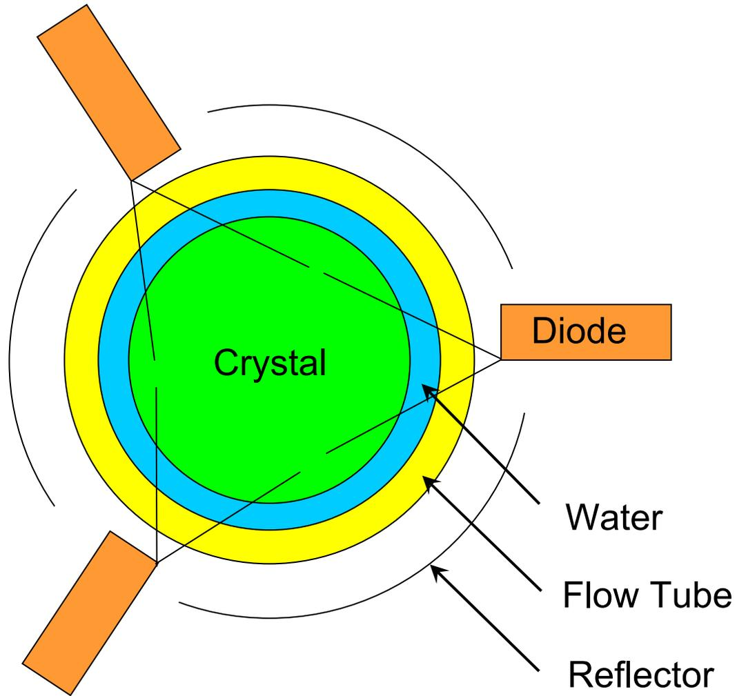
In this case the propagation of the pump beam in a plane perpendicular to the crystal axis is described by the Gaussian algorithm. It is assumed that the transformation of the beam traversing the different cylindrical surfaces can be described by appropriate matrices. This issue is described in more detail in Tutorial No.2.
