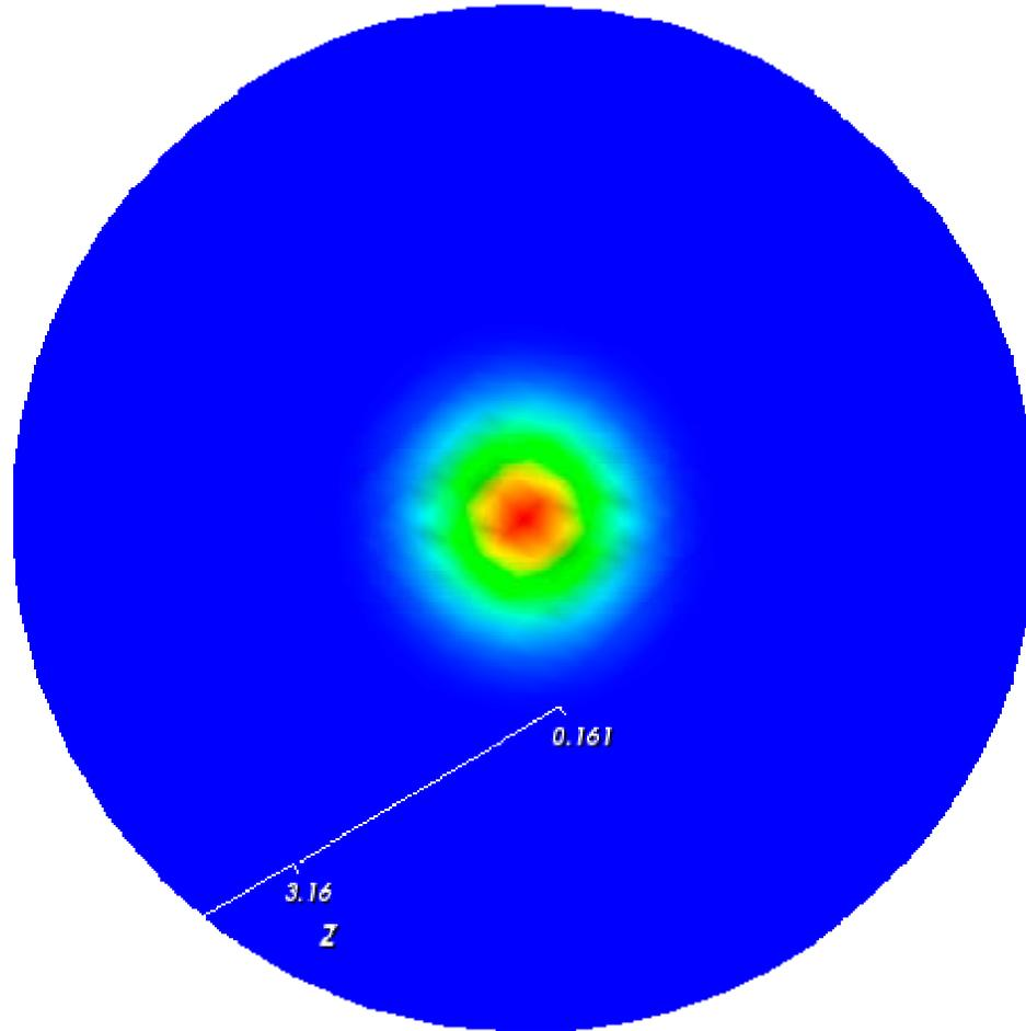
Beam profile for the same configuration with supergaussian aperture. Power output 4.22 W
