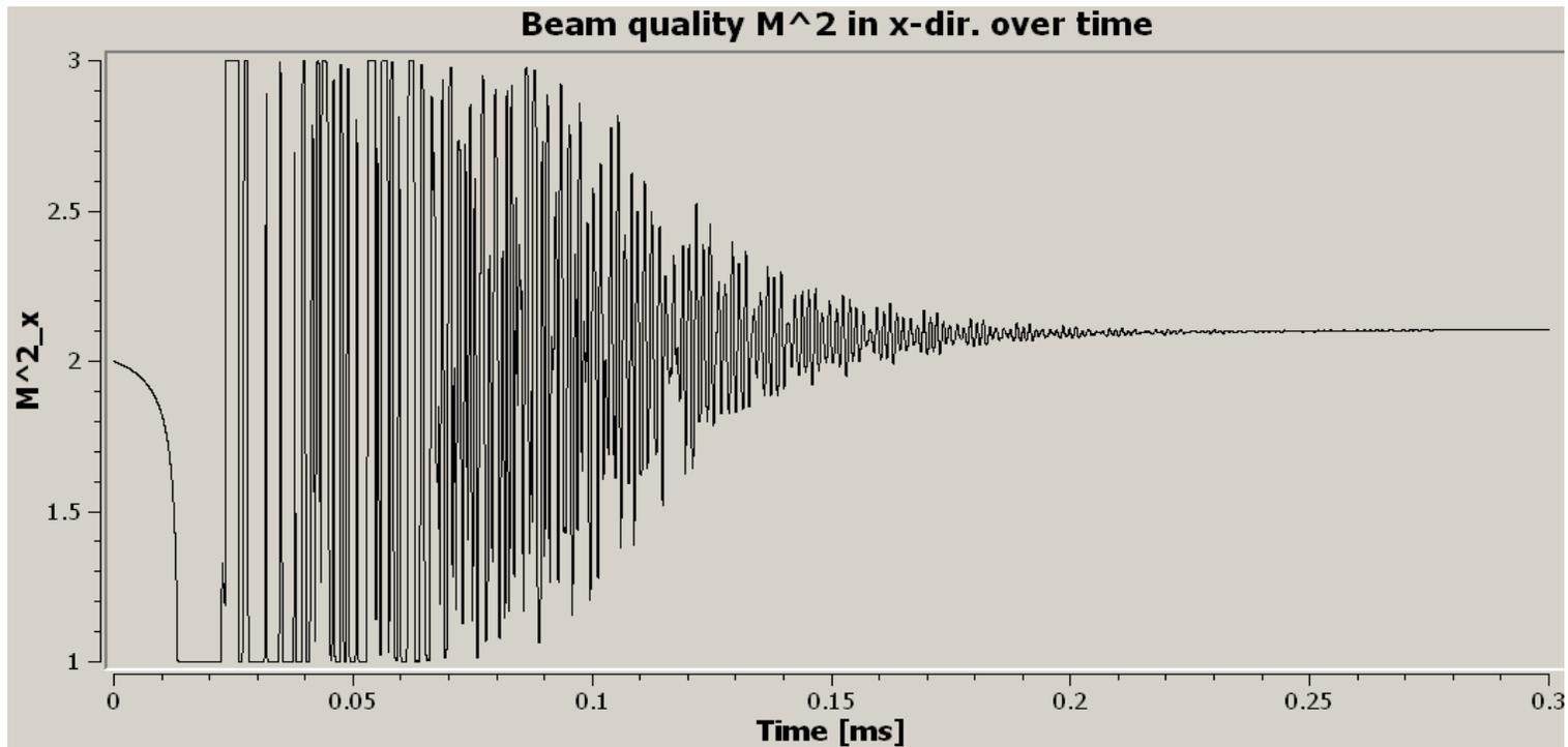
This plot shows a typical time dependence obtained for the beam quality.
