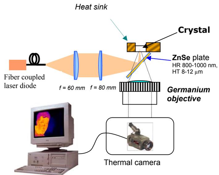
Figure 1. Experimental Setup
