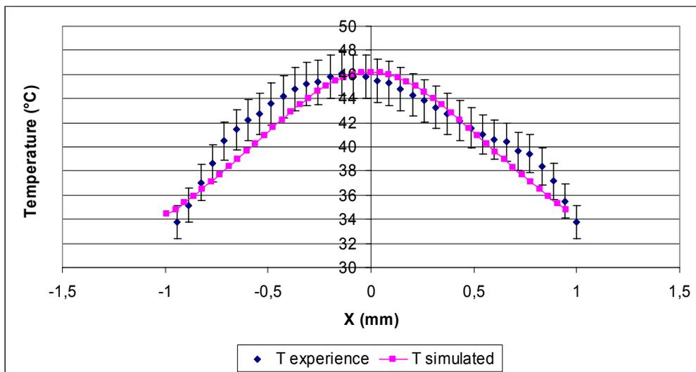
Figure 2. Measured and computed distribution of temperature T for Nd:YAG 1 at. % at the entrance plane of the pump beam.
