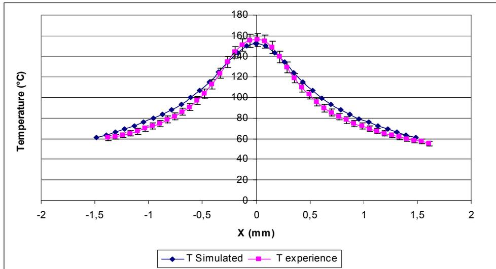
Figure 3. Measured and computed distribution of temperature T for Nd:YVO<sub>4</sub> 1 at. % at the entrance plane of the pump beam.
